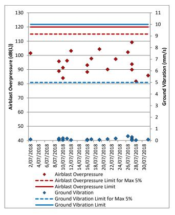
Figure 10: Moses Crossing Blast Monitoring Results – July 2018
