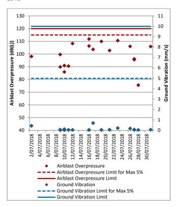
Figure 14: Knodlers Lane Blast Monitoring Results – July 2018
